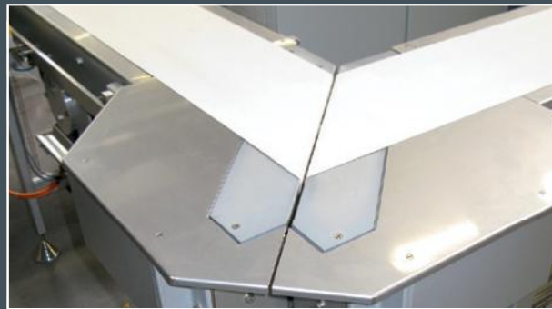
Cross feeding: Angular conveyors in tandem configuration for changing the product alignment
